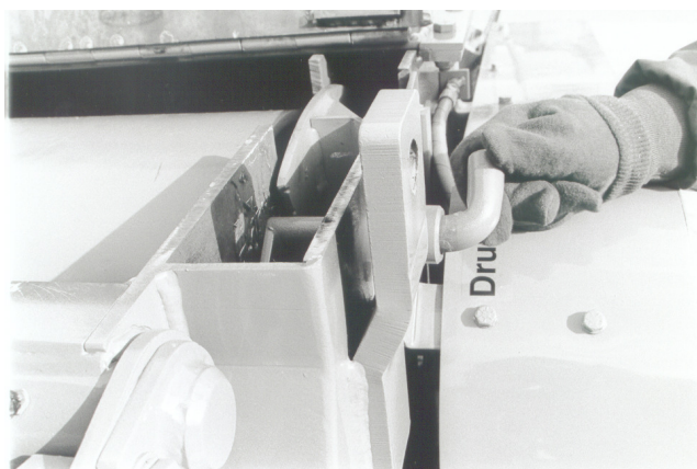
Drum Lock pin properly installed.
